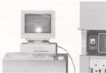
Computer controlled systems are available for HALT testing. The computer controller can operate up to three chambers.
