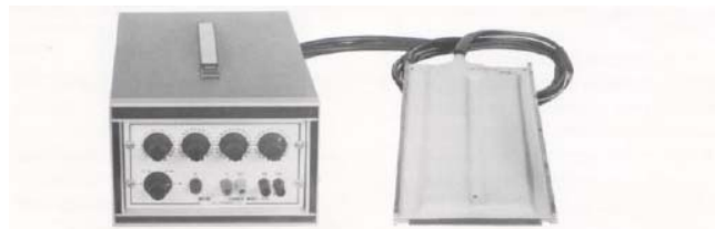
Manual Scanning Units allow the operator to connect the devices under test inside the test chamber to external test equipment.
